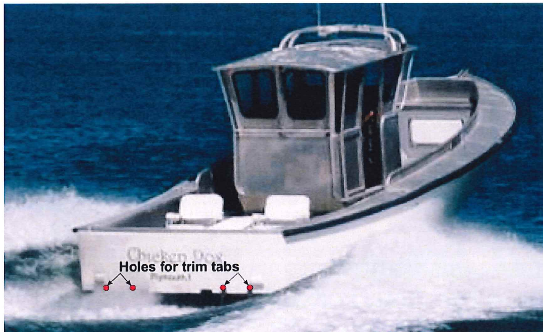
Figure 2. Trim tab hole location with boat in planing condition [photograph by Brian Woods http://downeastboatforum.com/free-classifieds-for-downeast-boats-marine-equipment-fishing-tackle-for-sale-or-wanted-/11236-31-jc-custom-aluminum-walkaround-pilothouse.html ]
